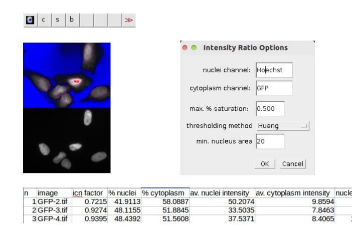
The tool calculates the ratio of the intensity in the nuclei and the cytoplasm. It needs two images as input: the cytoplasm channel and the nuclei channel. The nuclei channel is used to segment the nuclei. The measurements are made in the cytoplasm channel, after the background intensity has been corrected.
