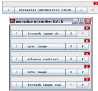
Figure 1. The tile representation of a simple application and its box representation. The applications is created by adding operations per drag and drop and by connecting them.
